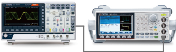
Direct Waveform Reconstruction from the DSO
