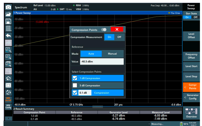
Measurement of 1 dB and 0.1 dB compression points
