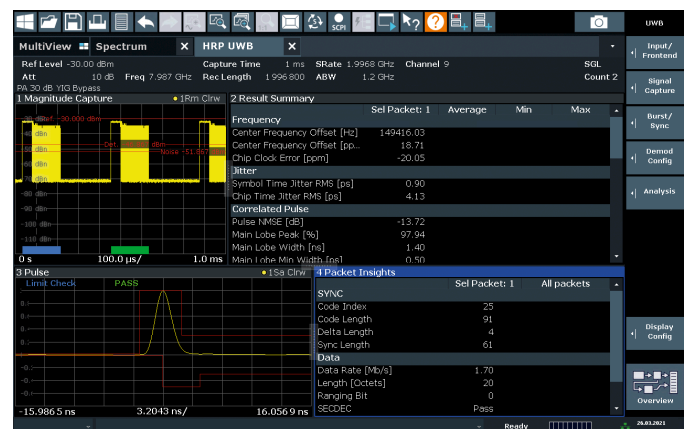
HRP UWB signal analysis with the R&S®FSW-K149 high rate pulse repetition frequency ultrawideband measurement application.
