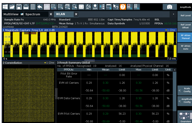
Analysis of a 320 MHz wide and 4096QAM modulated WLAN IEEE 802.11be signal using the R&S®FSW-K91BE option.
