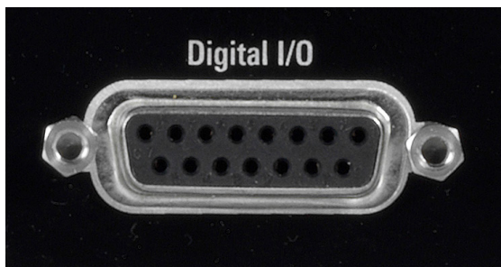
Digital I/O ports on rear panel
